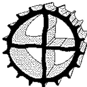
Figure 2. The KMT free-swimming carrier. Average size: diameter 11 mm, height 7 mm.
