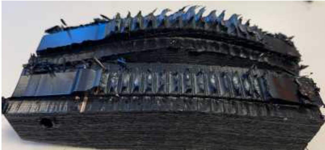
Duktilt brudd over, sprøbrudd under
