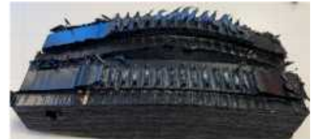
Duktilt brudd over, sprøbrudd under
