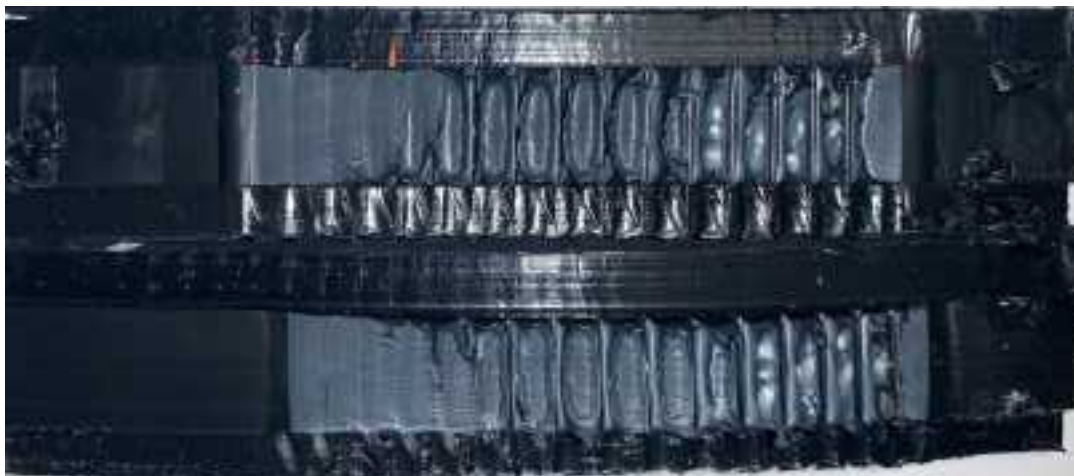
Duktilt brudd over, sprøbrudd under
